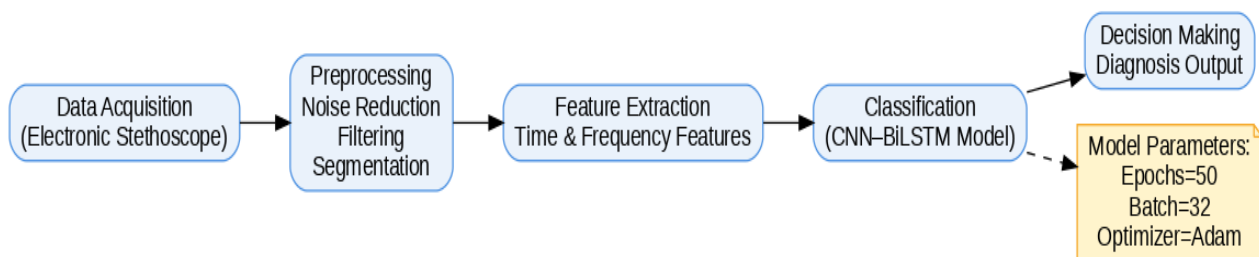
Figure 1. Heart sound processing and diagnosis process based on CNN-BiLSTM
