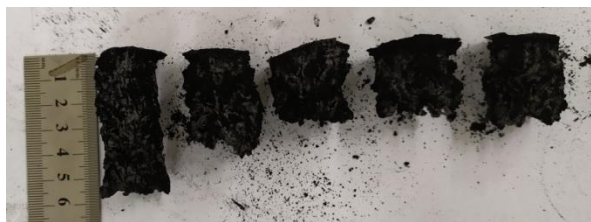
Figure 2. Carbon deposit, consisting of amorphous carbon, SWNTs and MWNTs.
