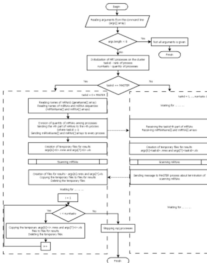
Fig. 1. Flowchart of the scanning program (parallel algorithm).
