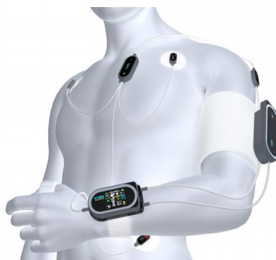
Figure 2. Visi Mobile is a body-wearable system of small sensors
